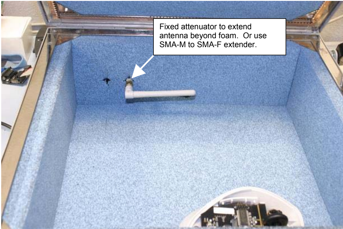
<Photo #2 – Fixed Antenna Mounting Example>
