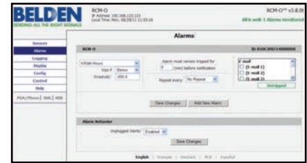
PDU Firmware, Alarm Setting Page
